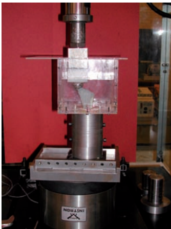
Evaluation of damage mechanism of CFRP femoral prostheses during fatigue testing using acoustic emission
