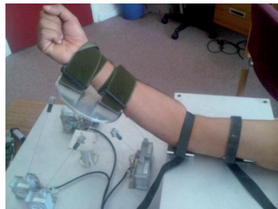
Stewart mechanism used in measuring 6dof joint mobility
