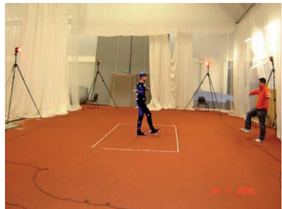
7 Cameras Eagle Digital Motion Capture System from MotionAnalysis, USA
