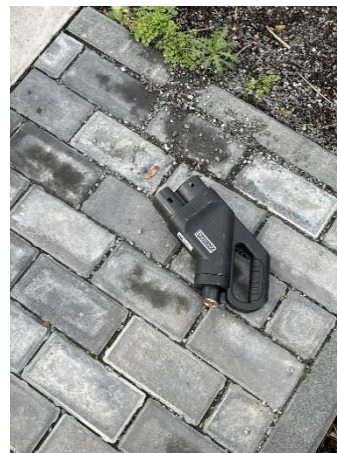
Figure 2: The abandoned CCS2 plug of a DCFC
