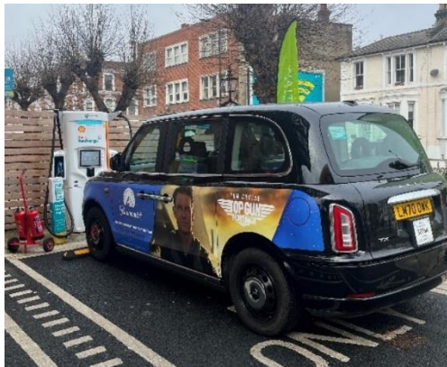
Figure 9: LEVC TX Taxi charging at a 350kW (capable) DCFC at a Shell Forecourt
