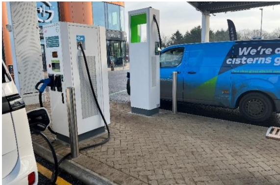
Figure 11: Vauxhall Vivaro-e operated by British Gas charging at a 350kW (capable) DCFC at a Gridserve Forecourt. In the foreground is a VW ID Buzz charging at a 90kW (capable) DCFC.
