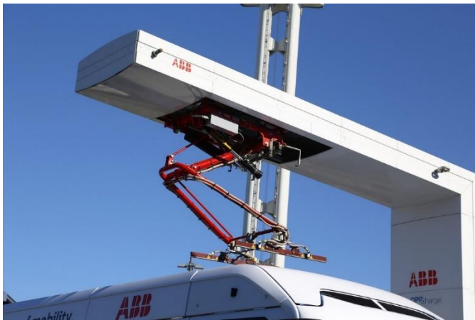
Figure 18: An ABB Pantograph automatically charging a bus. Source: ABB.
