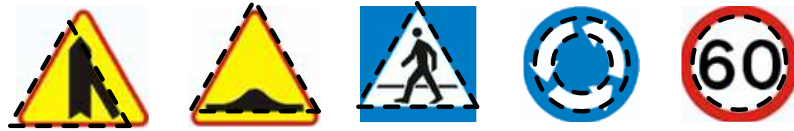
Figure 4.3: Examples of traffic signs where pictograms constitute extra regular shapes that are likely to confuse the circle/regular polygon detector. These shapes are marked with black dashed line.
