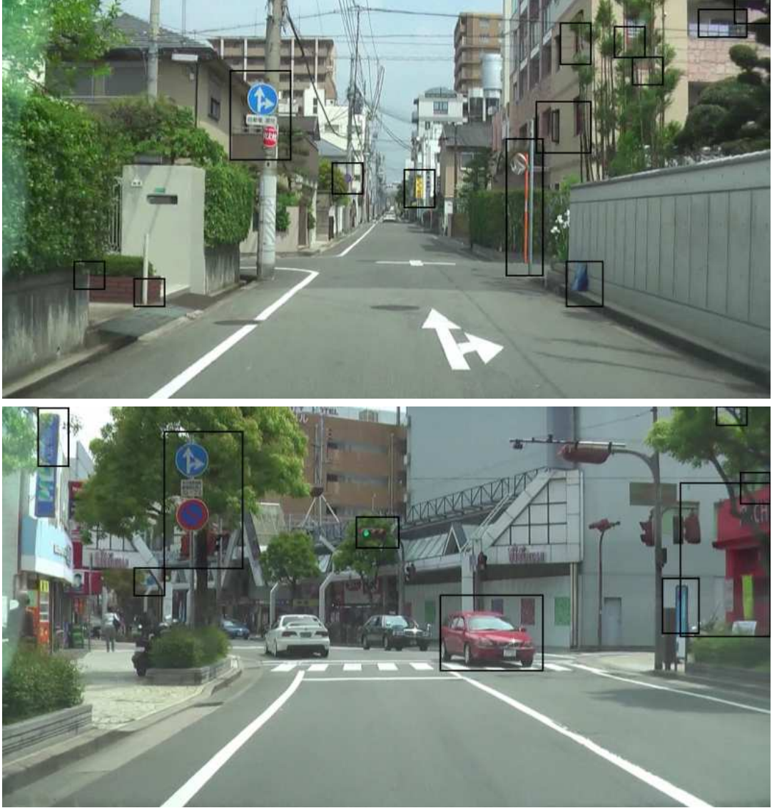
Figure 3.4: Example urban traffic images captured with a wide-angle camera mounted on board of a moving vehicle. On each image the regions of interest found by the proposed quad-tree focus operator are marked. The threshold t_{min} was set to the optimal value found in the training stage.
