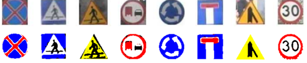
Figure 5.2: Example images obtained by the sign detector before (above) and after (below) background masking and colour discretisation; 2 bits suffice to encode colours in each image.
