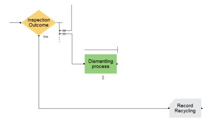
Firstly, we will add a **Record** module from the **Input Output** tab in the Project Bar. We do that in order to record how many products have gone for Recycling. This **Record** module will be connected with the **Else** output of the **Inspection Output**.
