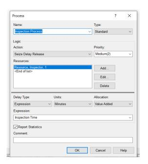
To configure the Inspection process, we double click it and then we put the values. We choose again "Seize Delay Release in the Action Tab.
