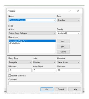
We double click on the **Process** module and we put the corresponding name on the **Name** Tab. Then in the **Action** tab we choose "**Seize Delay Release**". A **Resources** panel will show, on which we need to specify the Resource.
