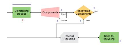
Then we will add a **Record** module and a **Dispose** module as we did in **Recycling** and **Refurbishment**.
