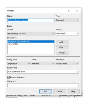
The Refurbishment process is set up as in the picture. As a Resource we add "RefTechnician" as it shows in the picture on the left. Pay attention to the Units, it should be Minutes!!
