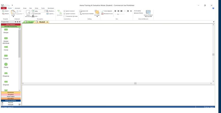
The main interface of Arena. On the right side of the screen (big blank box) is where you will build your simulation models. To build a model you need to drag and drop the processes from the Project Bar on the left side of the screen.
