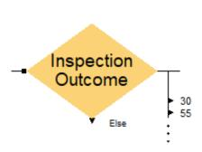
It can be seen that the percentages are shown for each decision and also there is an *Else* output on the module. As our percentages add up to 85%, there is still 15% left. This 15% is represented through the *Else* output. The 30% will be connected to the *Refurbishing* process, the 55% will be connected to the *Dismantling* process and the *Else* (15%) will be connected to the *Recycling* process.
