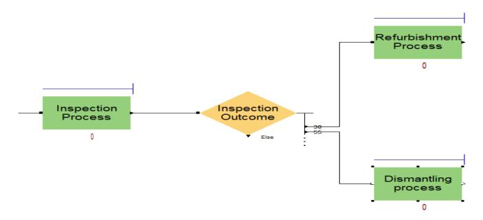
As it can be seen, we added two Process modules, one for *Refurbishment* and one for *Dismantling*. Pay close attention that each process is connected to the *Inspection Outcome* to its corresponding percentage.
