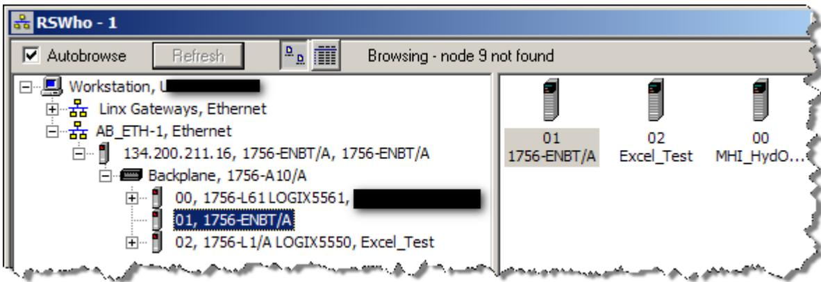
As you can see, I have a 10 slot CLX rack, with a 1756-ENBT card in slot 1 (address 134.200.211.16), and two processors, one in slot 0, and one in slot 2. The one in slot 2 is the processor we are going to use for this exercise.
