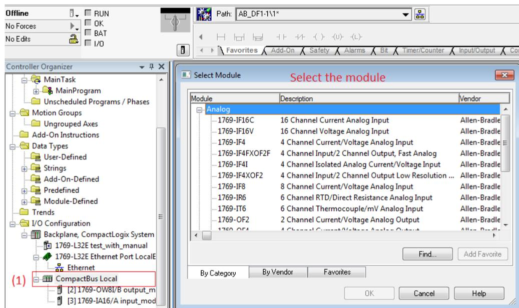
Figure 4. Configuring and adding modules to the project
