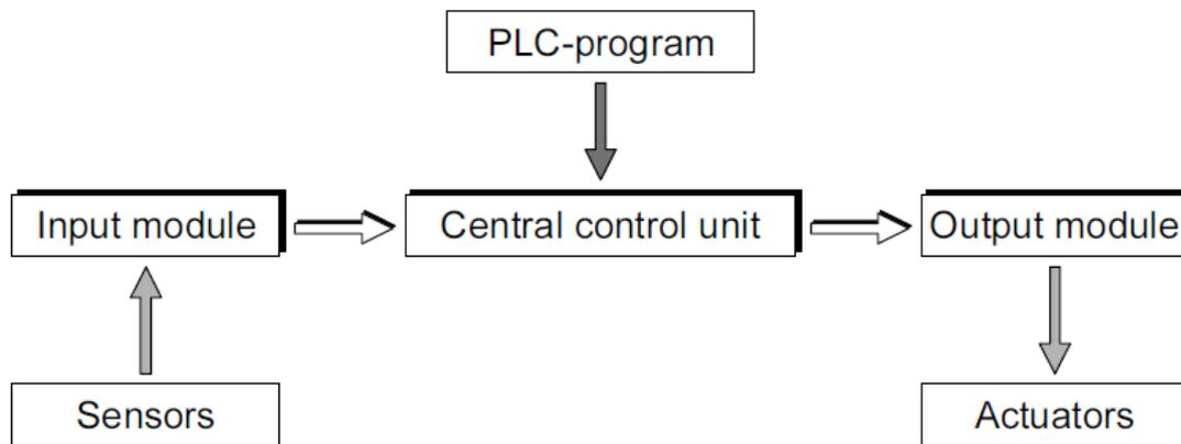
**Figure 1. PLC components**
