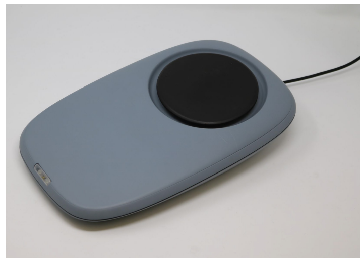
Upper casing with large movable foot controlled mouse
