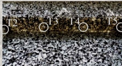
Thermocouples at fill interfaces
