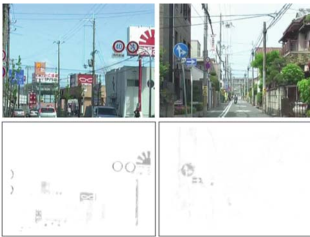
Fig. 2 The effect of applying the color filters (3) to the example RGB images (top row): red color filter (bottom-left), blue color filter (bottom-right)
